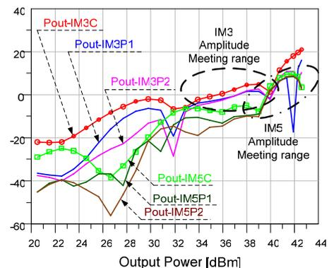
Figure 2. Two-tone simulations for IM3 & IM5 amplitudes of carrier and peaking amplifier
