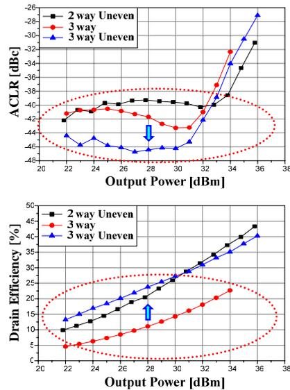
Figure 7. Measured ACLR and Drain Efficiency for WCDMA1FA signal
