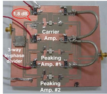
Figure 5. Implemented 3-way Doherty amplifier with uneven drive
