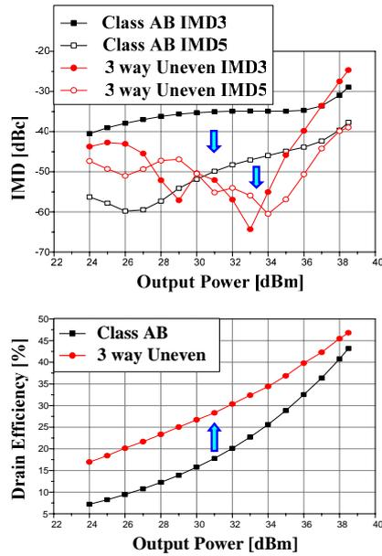
Figure 6. Two-tone measurements of IMD3, IMD5, and Drain Efficiency
