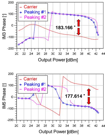
Figure 3. Two-tone simulations for IM3, IM5 phases of carrier and peaking amplifiers
