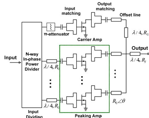
Figure 1. Block diagram of 3-way Doherty amplifier
