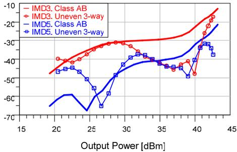
Figure 4. Two-tone simulations of IMD3 and IMD5
